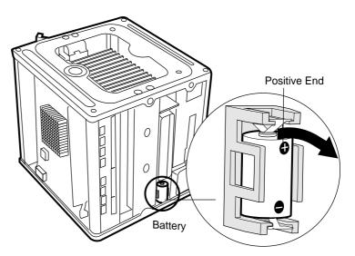
3 Insert the new battery into the holder, making sure the battery's positive and negative signs align with those on the holder.
